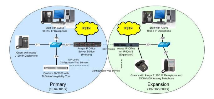
**Figure 1: Compliance Testing Configuration**
